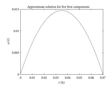
FIGURE 1: Approximate solution (26) of the governing differential equation in the elastic indentation phase for  $\beta = 1.9$ .
