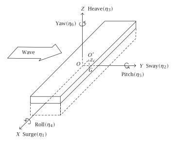
FIGURE 1.1. Sign convention for translatory and angular displacements of a floating body with the direction of wave propagation.
