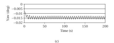
FIGURE 7.3. Time history of yaw motion for wave frequencies: (a) 0.56 rad/s, (b) 0.74 rad/s, and (c) 1.24 rad/s.
