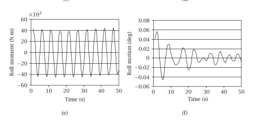
FIGURE 7.2. (a, c, and e) Time history of forcing function and (b, d, f) roll motion for wave frequencies (a, b) 0.56 rad/s, (c, d) 0.74 rad/s, and (e, f) 1.24 rad/s.
