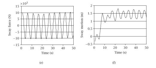
FIGURE 7.1. (a, c, and e) Time history of forcing function and (b, d, and f) sway motion for wave frequencies (a, b) 0.56 rad/s, (c, d) 0.74 rad/s, and (e, f) 1.24 rad/s.
