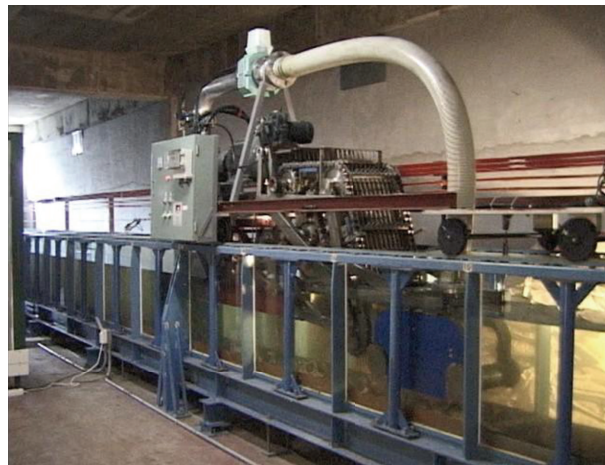
Figure 3: Test bed of hybrid type collector in 2-D flume.
