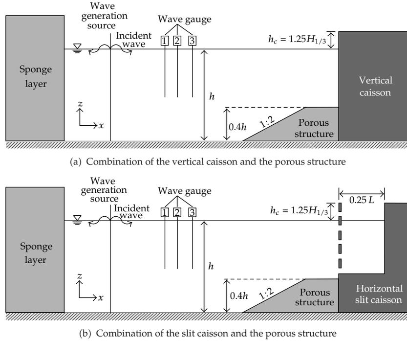
Figure 1: Schematic diagram of the numerical wave flume.
