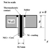
Figure 1. Schematic diagram of the set-up of the surface thermocouple (heat flux is experienced at the top surface)[1]
