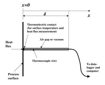
Figure 2. Schematic diagram of the set-up of the heat flux sensing pen
