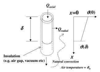
$Figure \ A.1.$  Schematic diagram of the heat flux sensor system for heat loss ratio calculations.
