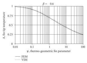
Figure 5.12. Variation of dimensionless fin tip temperature for  $\beta = -0.6$ .
