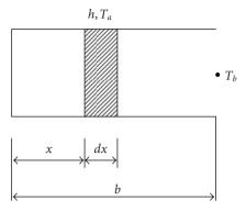
FIGURE 2.1. Geometry of a straight fin.
