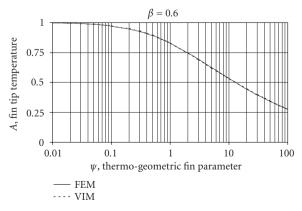
Figure 5.15. Variation of dimensionless fin tip temperature for  $\beta = 0.6$ .
