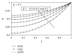
Figure 5.1. Comparison for dimensionless temperature variation for  $\psi = 0.5$ .
