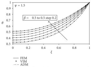
Figure 5.3. Comparison for dimensionless temperature variation for  $\psi = 1.5$ .
