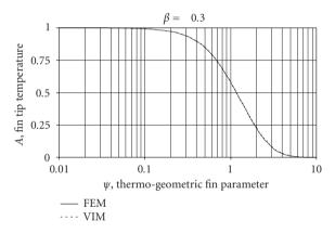
Figure 5.5. Variation of dimensionless fin tip temperature for  $\beta = -0.3$ .
