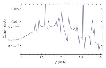
Figure 7: The induced current at Node 2 for a two-wire line in the cavity with an aperture.
