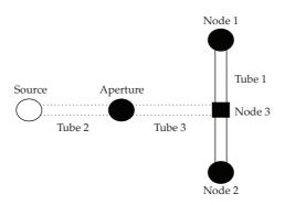
Figure 3: Topological network corresponding to the topological shielding diagram of Figure 2.
