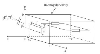
Figure 1: Cavity geometry enclosing a two-wire transmission line.
