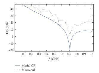
Figure 5: EFS for the empty cavity with an aperture by a plane wave.
