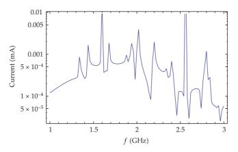
Figure 6: The induced current at Node 1 for a two-wire line in the cavity with an aperture.
