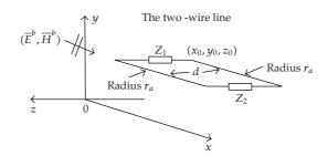
Figure 4: Isolated two-wire line excited by the interior field.
