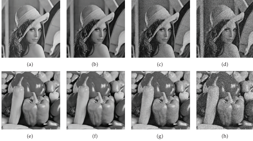
Figure 1: Multiplicative noise images. (a) Original “Lena” image; (b) image convolution with template 3 \times 3 of (a); (c) image with Gaussian white noise of mean 0 and variance 0.01; (d) image with Gaussian white noise of mean 0 and variance 0.05; (e) original “vegetables” image; (f) image convolution with template 3 \times 3 of (a); (g) image with Gaussian white noise of mean 0 and variance 0.01; (h) image with Gaussian white noise of mean 0 and variance 0.05.
