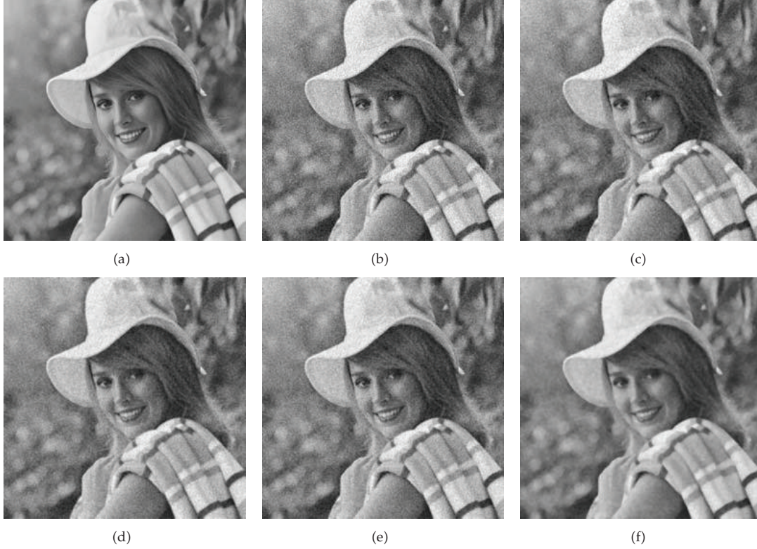
Figure 3: Detail of restoring noisy Elaine image ( 512 \times 512 ) with different filters. (a) Original image; (b) noisy image, PSNR = 20.0742; (c) median, PSNR = 26.4554; (d) averaging, PSNR = 27.6876; (e) wiener, PSNR = 26.7866; (f) TVM, PSNR = 30.0919.
