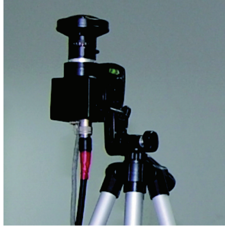
Figure 6: The prototype of the proposed visual sun compass.
